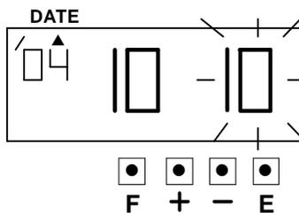
At the same time, the LCD screen only display “▲” under the “Date” mark.
