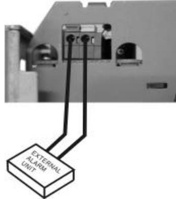
2. The connector for external time signal is on the back of the time stamp.
