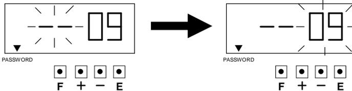
3. Press the [+] or [-] button to set the second two digits at [-], and then press [E] button. The display changes to the following figure.
