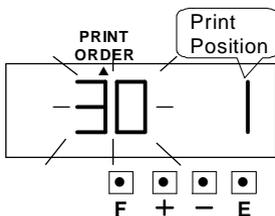
2. Press the [E] button. At the same time, the flashing digit changes from “Print Order Option” to “Print Position”.
