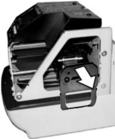
3. Turn the knob of the new cartridge in direction of the arrow (clockwise) to tighten the ribbon.
