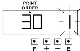
Such as example, press the [+] or [-] button to set at “1” and press [E] button, at the same time the LCD screen only display “▲” under the “Print Order” mark.
