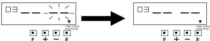
4. After you finished deleting the “Time Table Program”, press the [E] button again, the LCD screen will return to normal mode.
