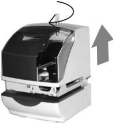
3. The two wires of external alarm unit, inset into the external time signal connector of time stamp.
