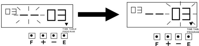
3. Press the [+] or [-] button to set at “-”, and then press the [E] button, the display changes to the following figure.
