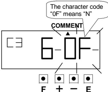
15. After you finished setting the customized comments, press the [E] button again, the LCD screen will return to normal mode.
