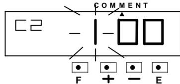
Such as example, the 1st character is “DATE”, press the [+] or [-] button to set at “28”, and press the [E] button.
