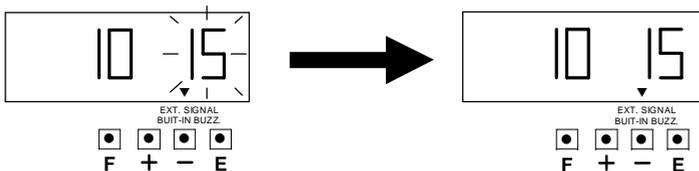
4. After you finished setting the external signal / built buzzer, press the [E] button again, the LCD screen will return to normal mode.
