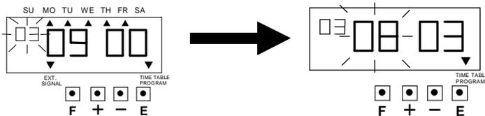
2. Press the [+] or [-] button to set at “-”, and then press the [E] button, the display changes to the following figure.
