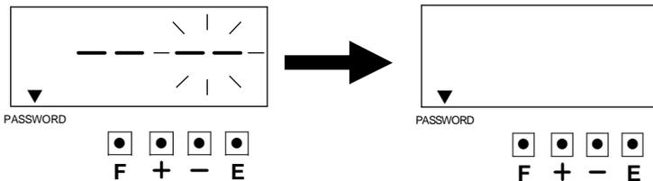
4. After you finished deleting the password, press the [E] button again, the LCD screen will return to normal mode.
