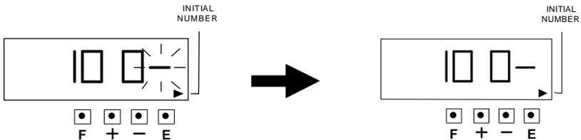
4. After you finished setting the Number, press the [E] button again, the LCD screen will return to normal mode.
