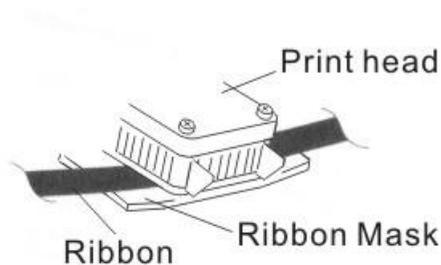
※**Notice:** install the ribbon cartridge so that the ribbon is between the print head and ribbon mask. Printing will not come out properly if the ribbon is placed behind the ribbon mask.
