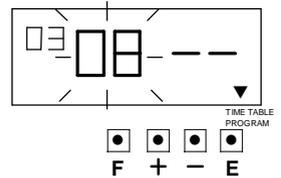
Such as example, press the [+] or [-] button to set at “8”, and then press [E] button. At the same time the flashing changes from “Code for Day of the week” to the “Code for Action”.
