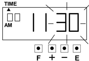
At the same time, the “Second” start to run from “00” and the LCD screen only display “▲” under the “TIME” mark.
