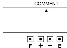
2. If you want to set another function, press the [F] button to continue setting. If you finished setting the functions, press the [E] button again. The LCD screen will return to normal mode.
