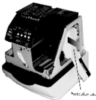
4. Plug the Ac cord into the Ac outlet and insert a card.
