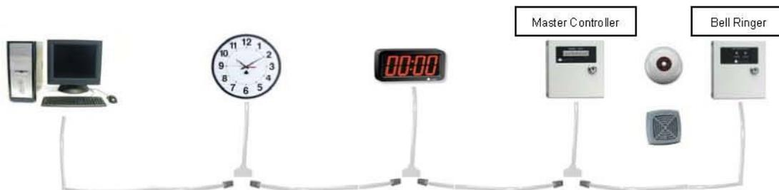
Figure 1: Model 7000 Master Clock & 4 Circuit Bell Control System
